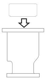
**Step Ten:** Replace lower float making sure that the lip on the float touches the baffle plate at the bottom of the valve and the Nozzle seat is facing upwards.
