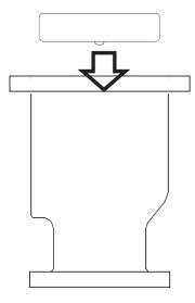
**Step Eleven:** Replace the Upper float/ small orifice float Making sure Nozzle is facing down and the flat face is facing up.
