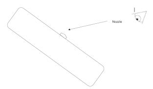
**Step Eight:** Checks the nozzle and ensure it isn't blocked or damaged if blocked clear with small wire. If damaged remove from float using a spanner and replace with Nozzle supplied in spares kit.
