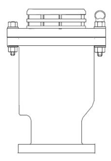
**Step Two:** Before removing the top flangeassembly ensure any excess pressure that may be trapped within the Valve body is be safely released ensure that the main Isolator is fully closed before doing this.
