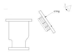
**Step Thirteen:** Check o'ring in top flange assembly for damage and replace with O'ring from spares kit if necessary.
