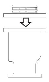
**Step Fifteen:** Replace top flange assembly making sure not to disrupt the O'ring groove.
