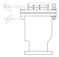
**Step Sixteen:** Replace nights and bolts nuts and bolts must be cross tightened.
