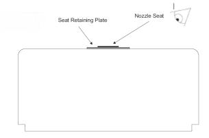
**Step Nine:** Checks the nozzle seat for damage if any damage is apparent replace with replacement seat from Spares kit supplied by manufacturer. In order to replace the nozzle seat Remove the Nozzle Seat retaining plate using a flat screwdriver to unscrew the screws and remove the Nozzle seat. Screw back the nozzle seat retaining plate once the new seat is in place.
