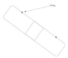
**Step Seven:** Check the O'ring on the "Anti-Shock float for damage replace with O'ring in spares kit if necessary.
