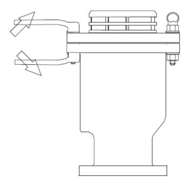
Step Three: Loosen nuts and bolts.
