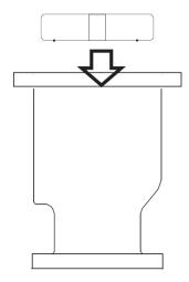
**Step Twelve:** Replace the "Anti-Shock" Float ensuring that the O-ring faces downwards and flat surface of the float faces upwards.
