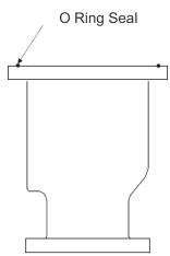
**Step Fourteen:** Check o'ring seal for damage and replace with spare O'ring Seal provided in spares kit if necessary. Make sure that it is properly placed in the groove before fitting Top flange assembly.
