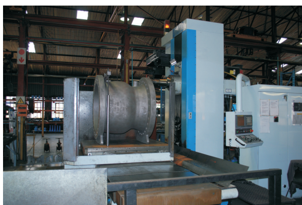
DN900 (36") PN25 NCV-B FLANGE MACHINING
