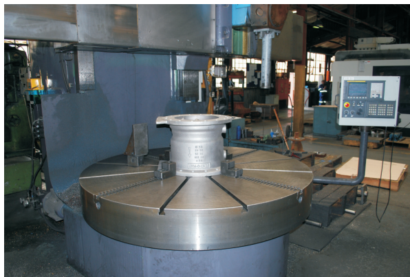
DN350 NCV- BODY SEAT MACHINING
