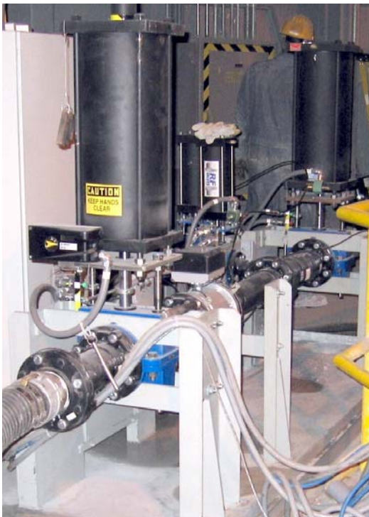
4" & 2" RF VALVE modulating w/digital control
